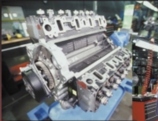
New "Moly" CNC machined engine blocks
