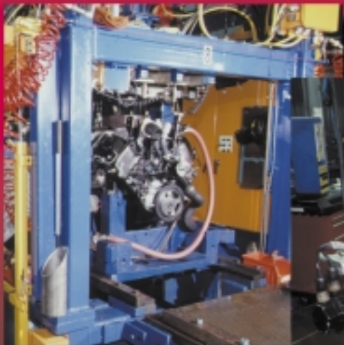
Total engine quality "Hot Test"
