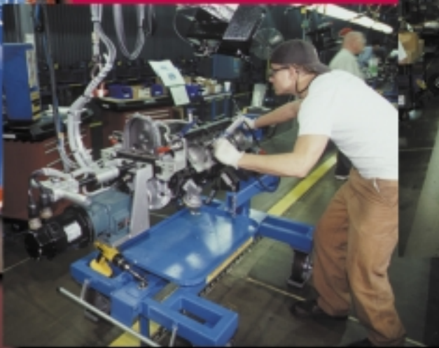
Computerized engine pressure check system
